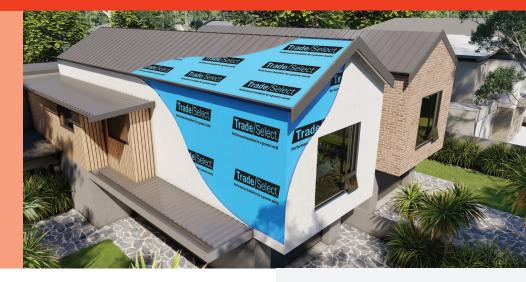
Trade Select™ FireSark® is an Extra Heavy Duty radiant barrier, designed for multipurpose use in all roof and wall types where fire performance is a priority. The reflective foil side provides extra R-Value when installed facing an air cavity, and the non-combustible glass fabric multi-layer structure provides excellent fire and ember resistance, as well as superior strength, flexibility and durability.
