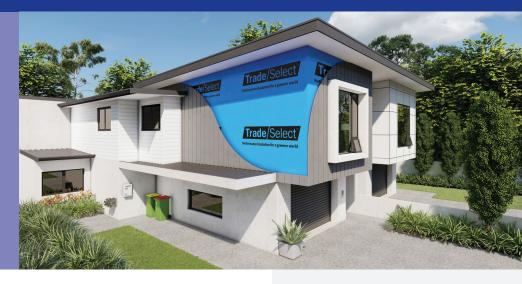
Trade Select™ VapourTech® Wall is classified as Air Barrier, Water Barrier and Class 4 Vapour Permeable. Very high levels of water vapour are allowed to absorb and diffuse through the core non-woven structure, ensuring that condensation risk is controlled, while outside liquid water cannot penetrate inwards. Trade Select™ VapourTech® Wall is chemically non-reactive in conjunction with treated timber and salt conditions close to coastlines.
