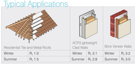
Typical Residential 22° Pitched Tile / Metal Roof with one layer of Trade Select FireSark™ CALCULATION REFERENCES: Tile Roof 299r38fs / Metal Roof 299r37fs. Typical Aluminium Composite Panel Wall ACP/Lightweight Cladding fixed to battens with one layer of Trade Select™ FireSark™ fixed to 90mm stud, R2.5 fibrous insulation & 10mm plasterboard CALCULATION REFERENCE: 299w40fs. Typical Brick Veneer Wall with one layer of Trade Select™ FireSark™ and R2.5 insulation CALCULATION REFERENCE: 299w39fs.
